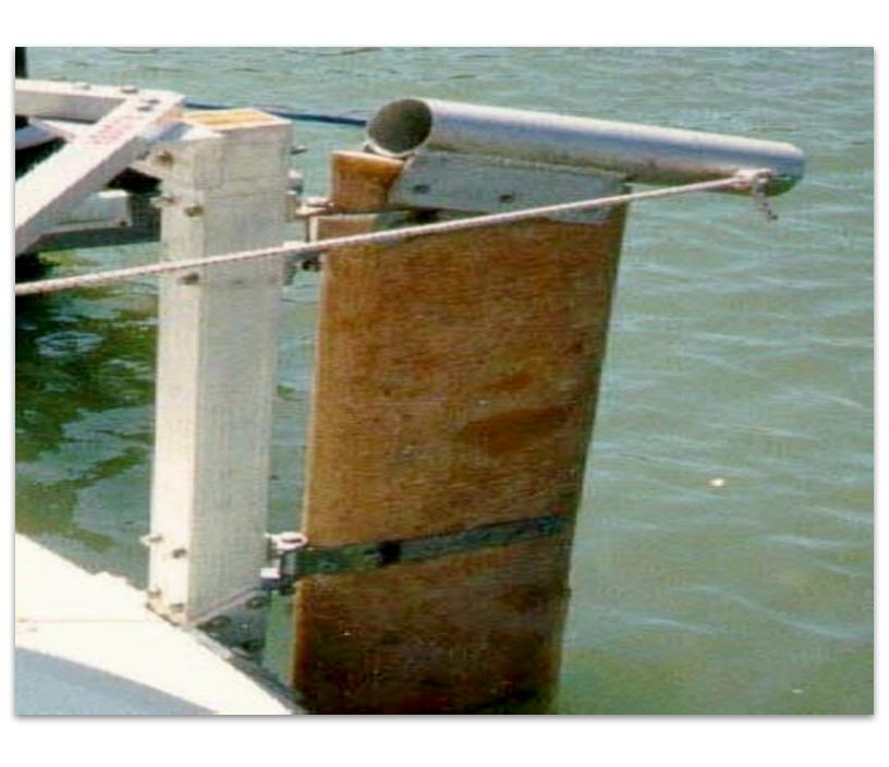
Hanging off the back of the boat to install this rudder in any sort of sea state would be difficult and dangerous.
