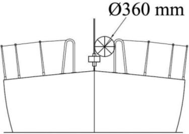
Figure 2 - Diagram Showing Pulpit Opening
